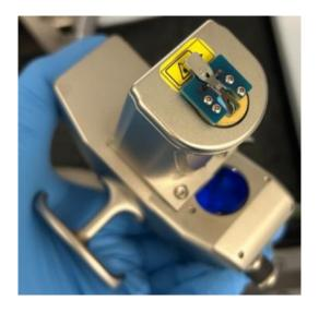
e) Carefully flip the scanner back over and return it to the slot. Lower it slowly until reach the bottom— the top of the scanner should align with the black reference line on the mounting post — then tighten the screw back.
