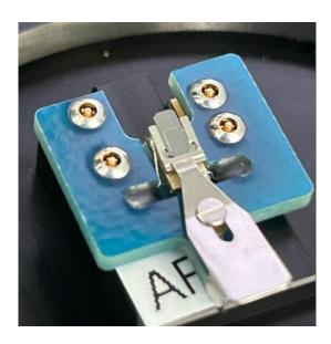
d) Push the clamp down and then forward so that it holds the probe in place
