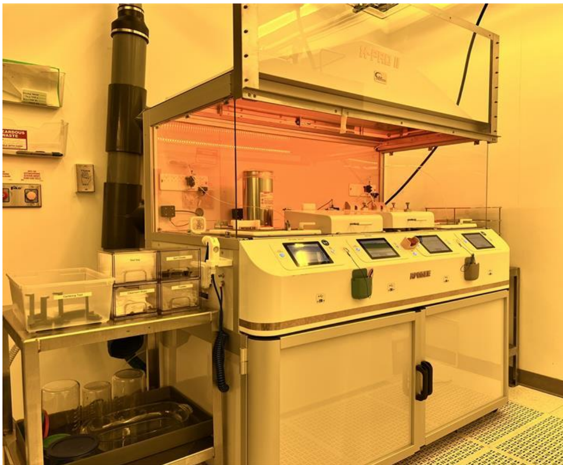
Figure 1. Apogee spin coater, bake plate, vapor HMDS bake plate system in Bay 4, Aggiefab.
