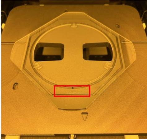
**⚠ Warning!** The operator should be able to read “TOP” in the frame highlighted in the image above. If it is inverted, then the orientation of the quartz plate is wrong! This quartz plate is **fragile and expensive**, once it has a crack, it cannot be function anymore, please contact Aggiefab member for the use in your wafer bond aligner session and return it back when you session is over.
