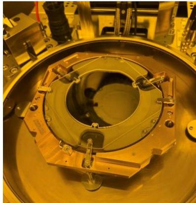
Step 28: **“Move Tray out”** → Pull the tray out completely.
