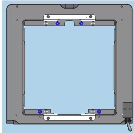
**⚠ Warning!** Check all **four o-rings** are present. Missing o-rings can compromise alignment.
