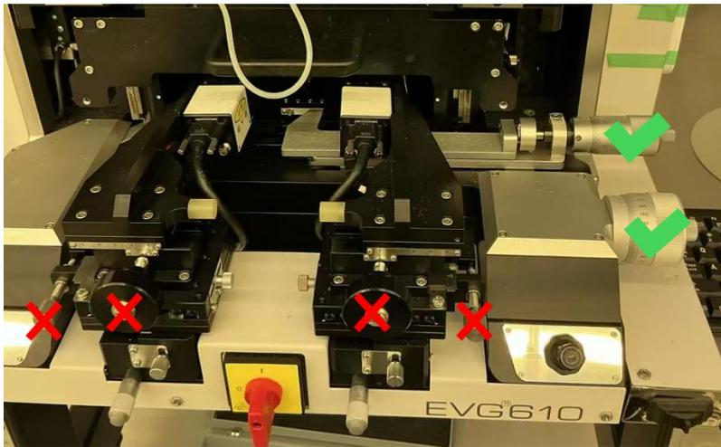
**Step 23: "Align Substrate"** → Align wafer2 with the crosshair. Repeat the alignment as in the previous step.
