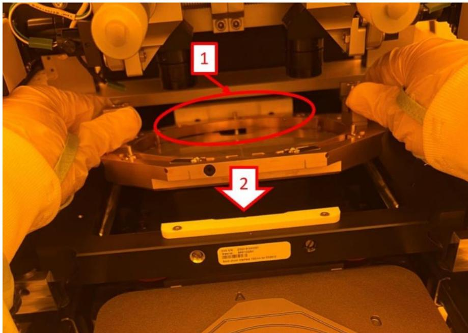
Step 6: "Remove Clamps" → Rotate the clamp knobs as depicted in the animation.
