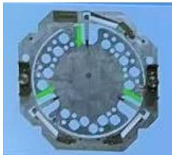
Step 26: **“Insert Clamps”** → Insert clamps as shown in the animation. Make sure to push the clamp knobs all the way down in order not to touch the quartz plate during rotation. **Try to release the knobs simultaneously on both clamps. If done properly this action should not induce any loss of the fine alignment.**
