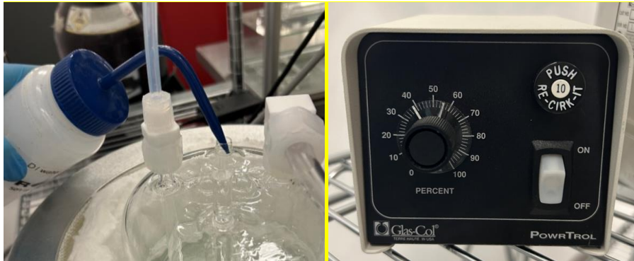
Figure 2: Filling the Bubbler (Left) & Bubbler Power Control (Right)
