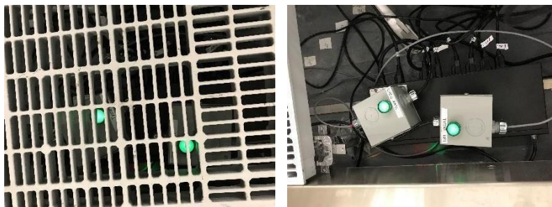
Figure 1. Interlock box under subfloor, showing tool ON iLab status.
