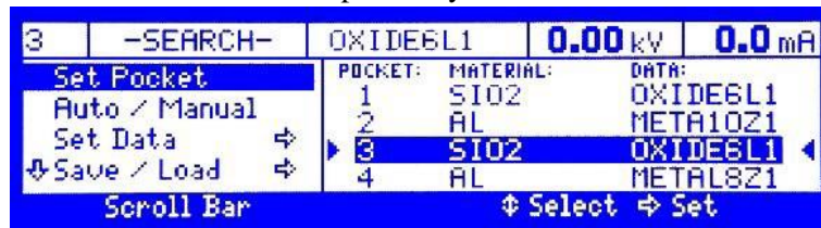
Fig. 3: EB gun controller screen. Left joystick controls “Set Pocket” and “Auto/Manual” (left side) and right joystick controls the Pocket/Material/Data (right side).
