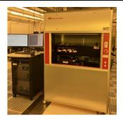
The Heidelberg MLA 150 Maskless Aligner is a highspeed direct laser writer for photolithography without contact on a substrate. It utilizes diode lasers and a high-precision stage to write the laser on a substrate from design files, which enables rapid prototyping of tiny features and photomask generation.
