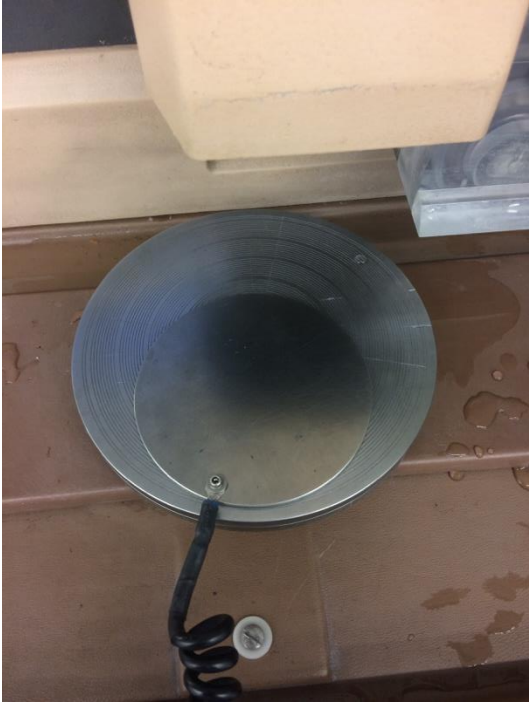
Figure 3: Correct placement of gauge block for chuck zeroing.
