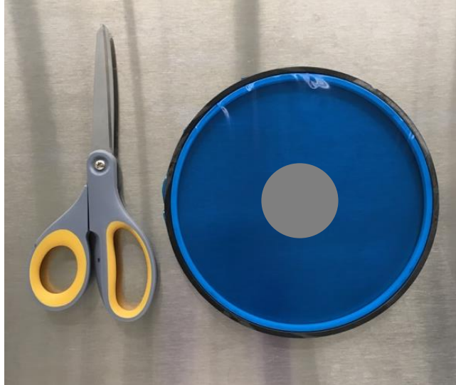
Figure 1: A wafer placed on the blue tape with excess tape cut off.
