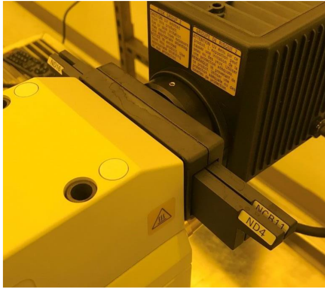
Figure 15. Apertures located at the back of the microscope. Note the even spacing.
