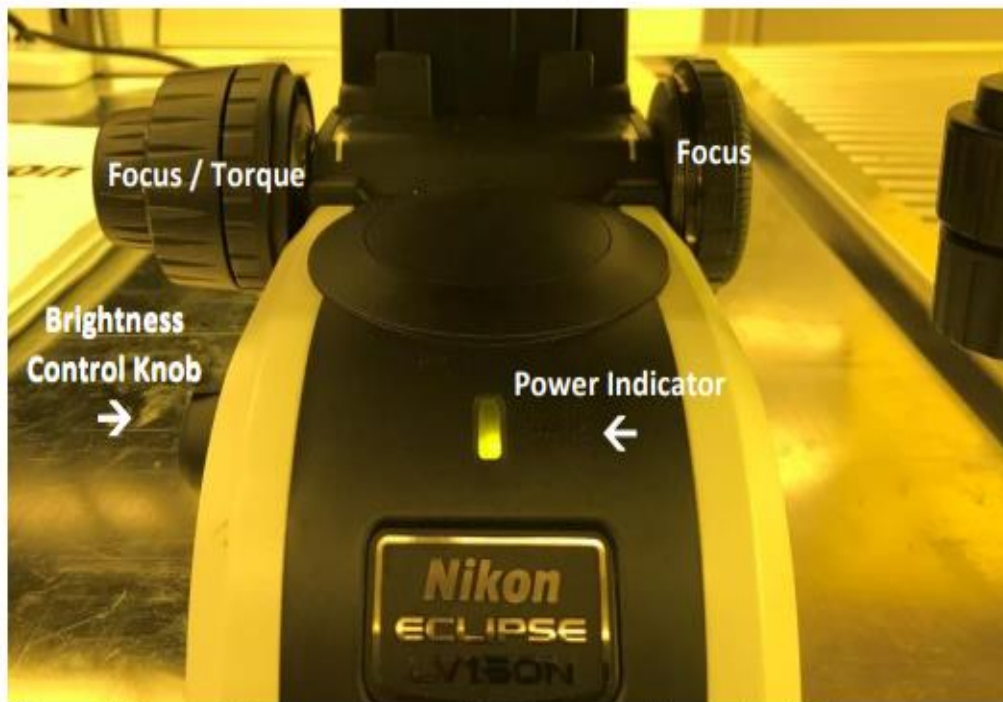
Figure 1. Power indicator at bottom of microscope and lower-level adjustments.
