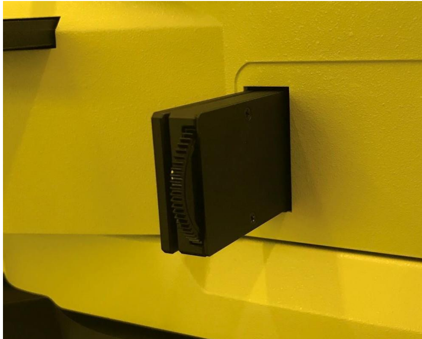
Figure 17. Aperture located on the right side of the microscope above the objective lenses. This is in a middle position that the aperture “clicks” into.
