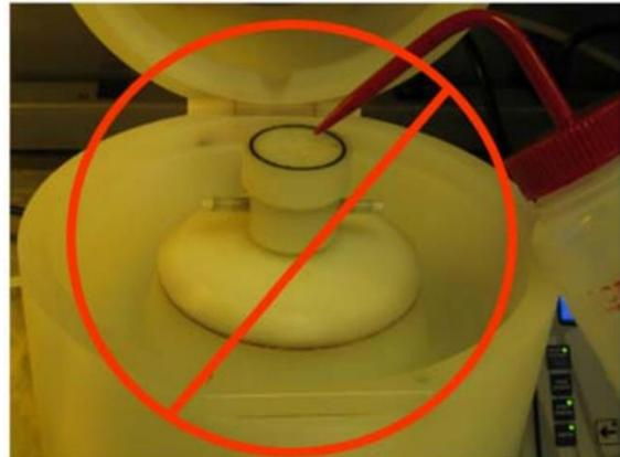
Please DO NOT force any liquid or compressed air into the vacuum path
