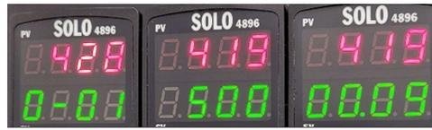
Figure 8. Control panel showing step number (left), set temperature (middle), and time remaining (right).
