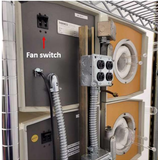
Figure 2. Fan switch on the back of furnace.
