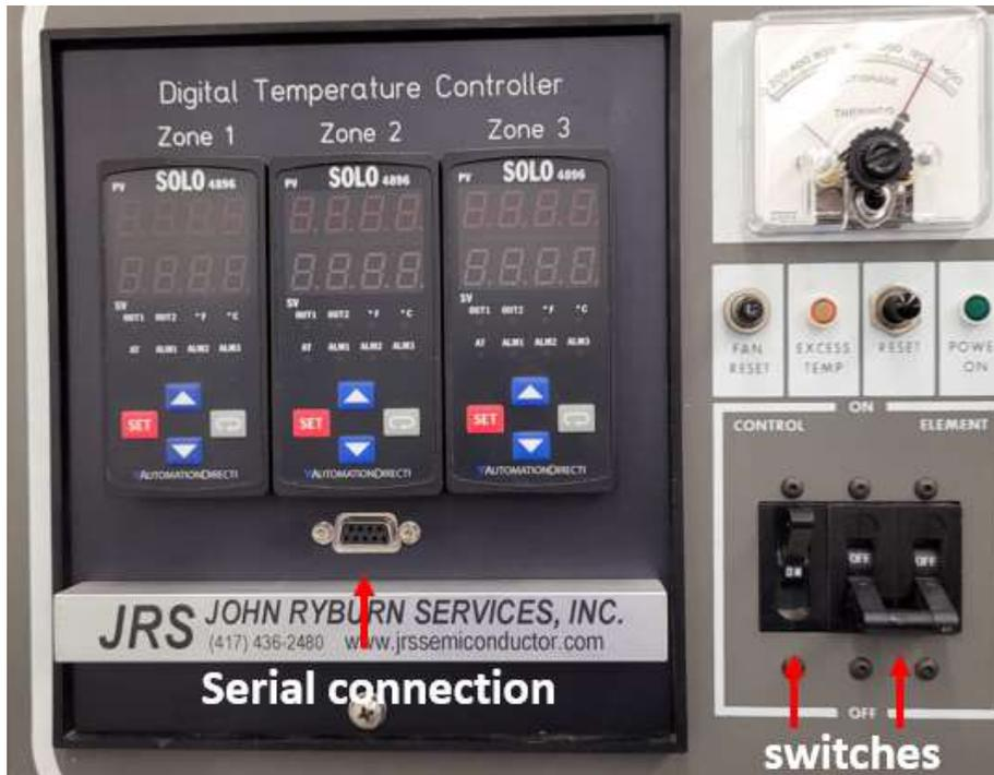
Figure 3. Controller & heating element switches.
