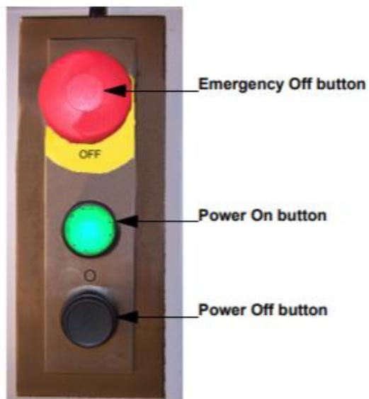
Figure 2: Power On/Off Switch Panel (The tool can still be on without the “On button” being lit)
