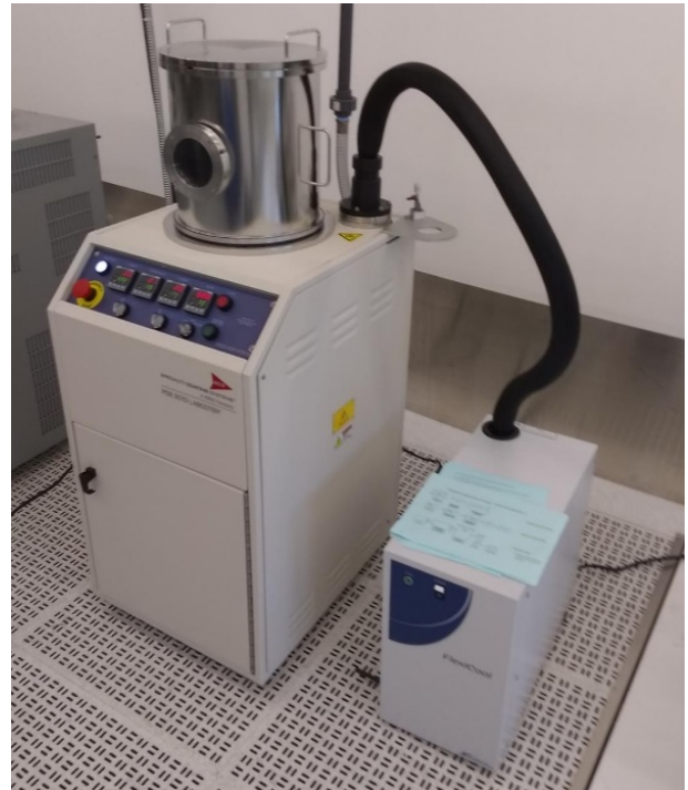
Parylene setup w/ top chamber (left) and Mechanical Chiller (right)
