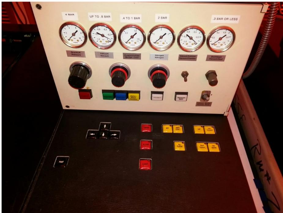
Notable components: Separation and Kontakt lights (green and blue), Expose, Align, and Load buttons, arrow keys to move aligner and microscope for viewing purposes, and mask vacuum switch.
