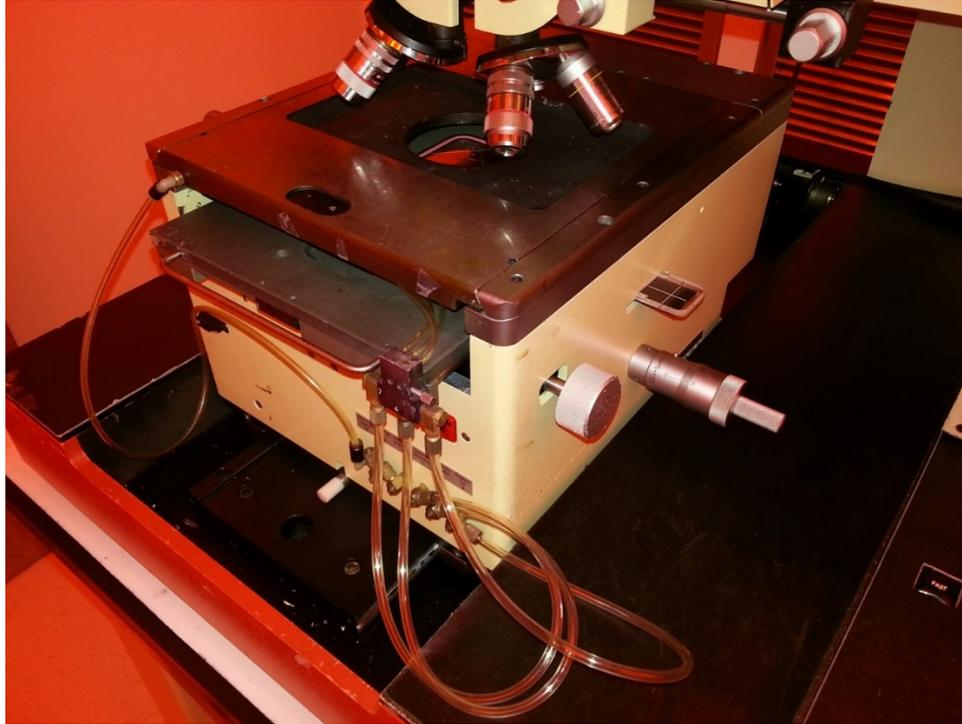
A view of the X-axis control knob, the Theta control knob, and the alignment guide.
