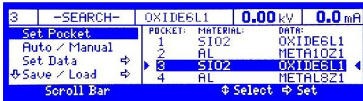
Fig. 5a. Crucible pocket selection for hand held e-gun controller.
