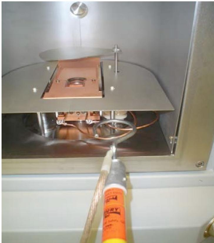
**Fig. 1. Use of grounding rod on e-gun electrodes.**
