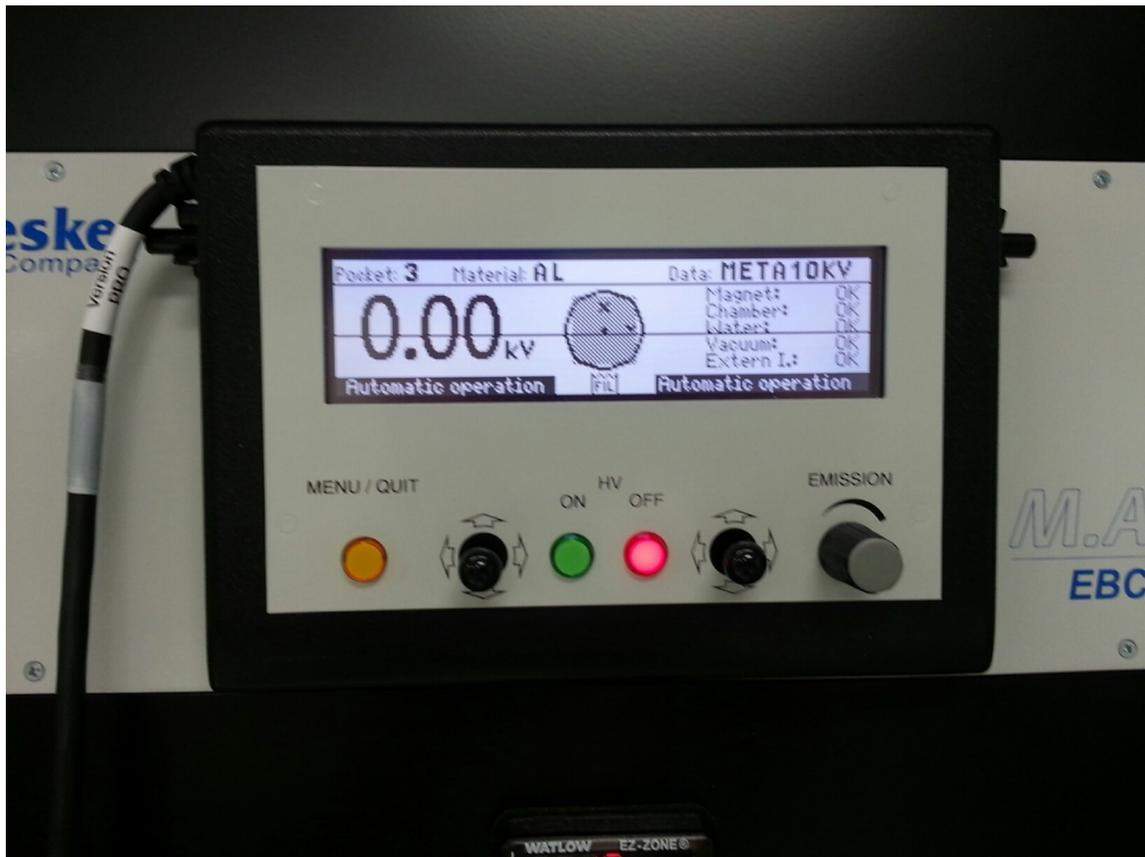
Fig. 4. Hand held E-beam controller is located behind the right side door.
